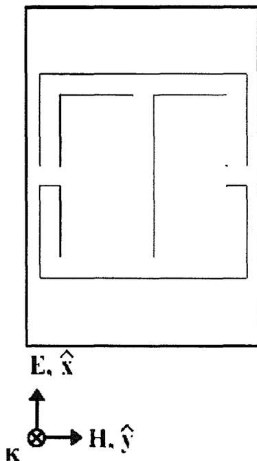
**Figure 2. Example of Another Metamaterial Component: Electric Ring Resonator (ERR).** This component provides tunable resonant electric response to the incident electromagnetic field, and can be utilized for engineering the frequency-dependent dielectric permittivity  $\epsilon(\omega)$ . Possible application: THz and microwave absorbers. (Reference 7)
