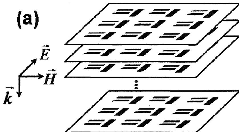
**Figure 17. True Multi-Layer Metamaterial With a Unit Cell Shown in Figure 15:** radiative antenna (single metal strip) coupled to a dark antenna (two perpendicular metal bars). Such metamaterial exhibits "slow" light propagation along the incidence direction (slowed down by a factor 30 or more). (Reference 32)
