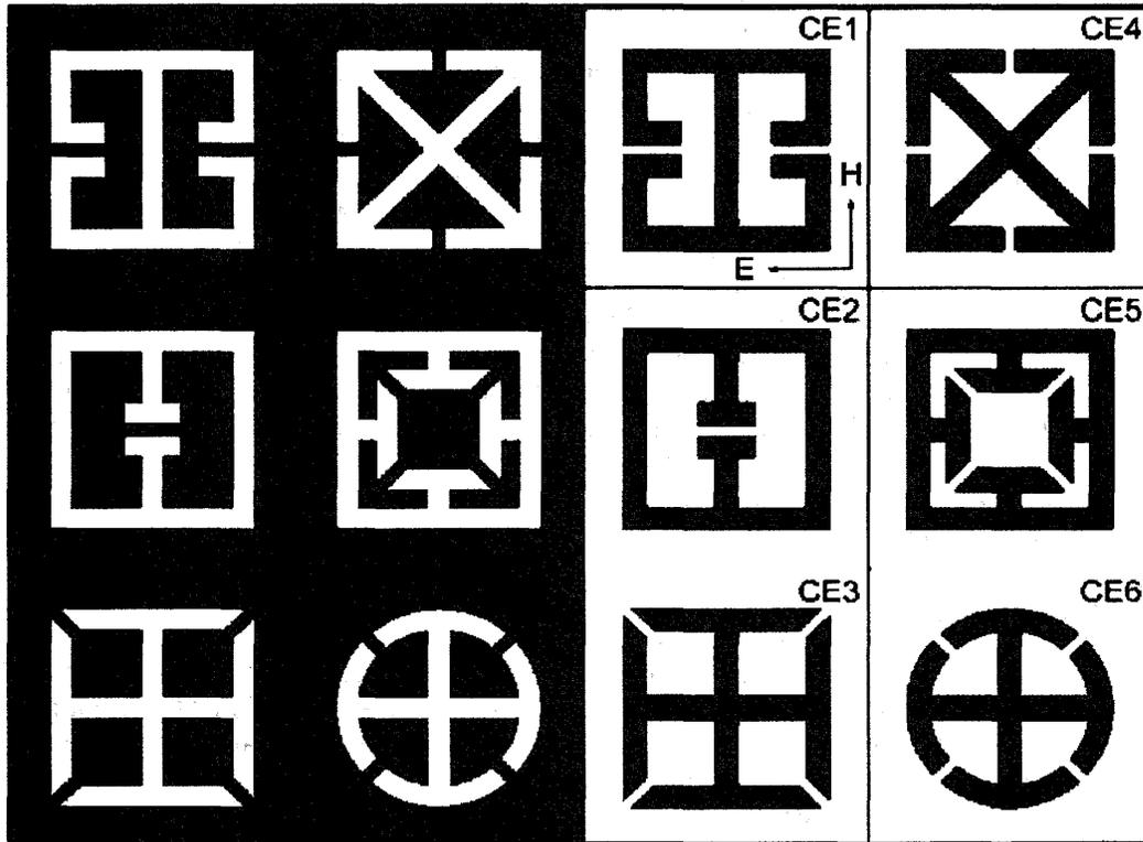
**Figure 3. Geometry of Original Planar Metamaterial Unit Cells (OE1-OE6) and Their Complements (CE1-CE6).** The polarization of normally incident electromagnetic radiation is configured as shown in OE1 and CE1 for the original and complementary metamaterials, respectively. (Reference 9)
