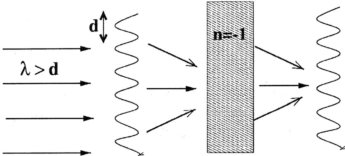
**Figure 5. Schematic of the Super-Lens with  $n=-1$  Refractive Index Corresponding to  $(\epsilon = -1, \mu = -1)$  Surrounded By Vacuum.** Super-lens' presence enables imaging sub-diffraction objects such as the periodic grating shown here.
