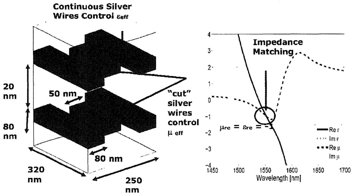
**Figure 20. Specific Design of a Wide-Angle Plasmonic Absorber Based on Negative Index Metamaterial Operating at  $\lambda=1550$  nm.** Left panel: Schematic of the silver-based plasmonic structure. Right panel: Extracted permittivity and permeability for the normal incidence demonstrate impedance matching:  $\epsilon_{yy} = \mu_{zz} = -1 + i$ . (Reference 20)
