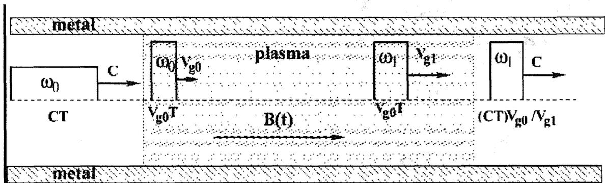
**Figure 14. Schematic of Pulse Compression in Magnetized Plasma.** A radiation pulse with initial frequency  $\omega_0$  and duration  $T$  slows down in the plasma to a group velocity  $v_{g0} \ll c$ . Adiabatic spatially uniform variation of the magnetic field changes the radiation frequency to  $\omega_1$  and increases the group velocity to  $v_{g1} \gg v_{g0}$ . The emerging pulse is compressed to  $T_1 = T v_{g0} / v_{g1}$ . (Reference 29)
