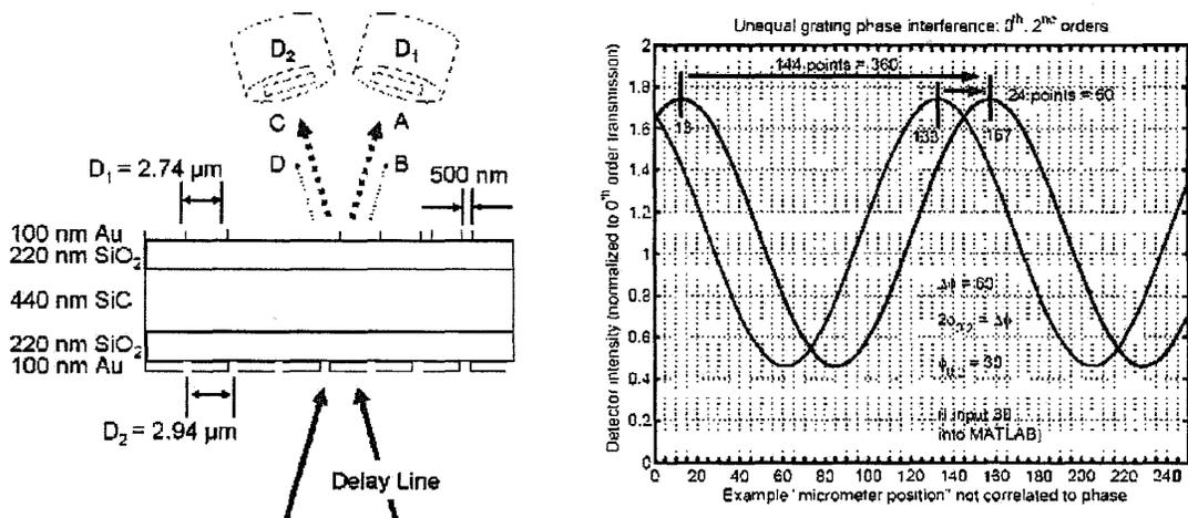
**Figure 12. (Left): Schematic for 2-Beams/2-Detectors Interferometric Measurement. (Right): Numerical Simulation:** intensity on the two detectors as a function of the phase delay between beams A and B produced by the interference between the zeroth and first diffractive orders of the bottom diffractive grating (numerical simulation). The second detector provides the necessary second data point which is necessary for separating the contributions of different diffractive orders.
