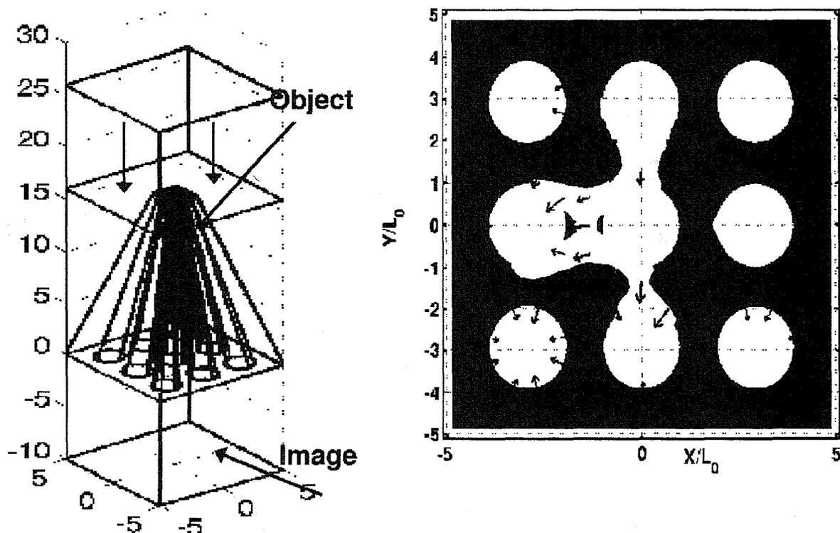
**Figure 8. Hyper-Lens Based on a Converging Array of Metal Wires.** A small object can be placed at the tip, illuminated from the top, and magnified by the expanding array of wires. Left panel: schematic. Right panel:  $\lambda/25$  object magnified by a factor 5x by the expanding hyper-lens. This hyper-lens can operate at mid-IR frequencies. (Reference 26)
