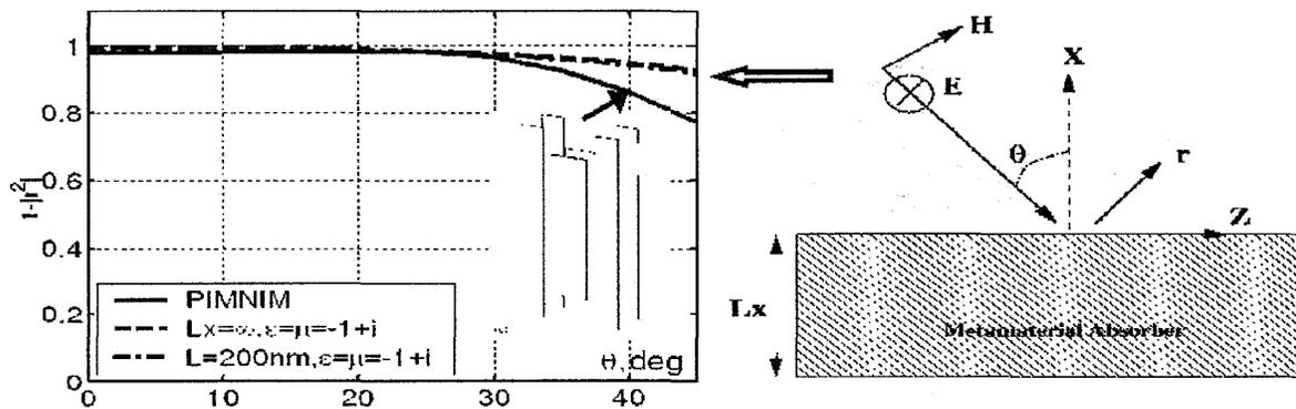
**Figure 19. Wide-Angle Plasmonic Absorber Based on Negative Index Metamaterial.** Right panel: schematic of an absorption-measuring experiment. A generic metamaterial with  $\epsilon_{yy} = \mu_{zz} = -1 + i$ ,  $\mu_{xx} = 1$  is assumed. Left panel: angular dependence of the absorption for a generic and specific (shown in the inset) metamaterial. Both exhibit wide-angle absorptivity. (Reference 20)
